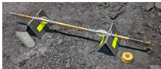
*Centralizer blades mounted on running gear*
